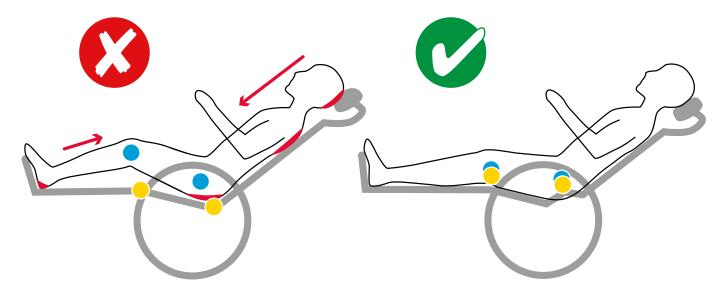
Weight shifting has been built into the Rea chairs to ensure the wheelchair is stable no matter which seat angle the chair is at. In basic terms, it allows the seat to move downwards and forwards which enables it to retain its stability, despite the backwards leaning position. The seat simply slides towards the chassis.
