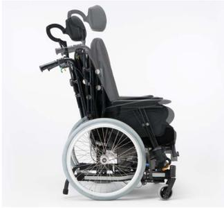
The first 10° of **Dahlia** 30° has a small incline for keeping the feet as close to the ground as possible.
