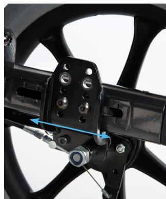
The centre of gravity can be adjusted for lighter wheeling.
