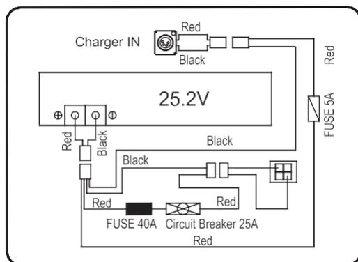
Lead-acid battery - Circuit diagram
