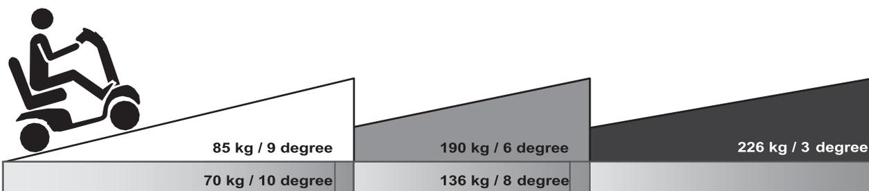
The grade climbing degree will be affected by weight capacity, driving speed, and ramp degree, and scooter parameter. To prevent any danger from a defected motor, please avoid to drive on long ramp or any uneven terrain.
