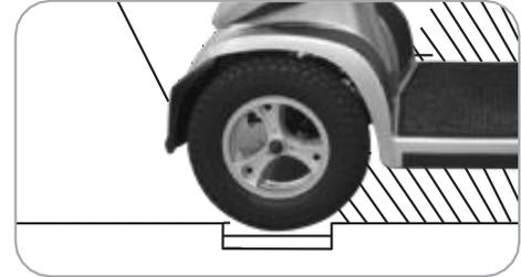
When driving scooter on ramp, adjust body centre of gravity to keep scooter safer.
