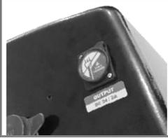
The DC 24/2A port is for LED reading light use ONLY. Do not use the port to charge scooter or any other devices. (For 928C only)
