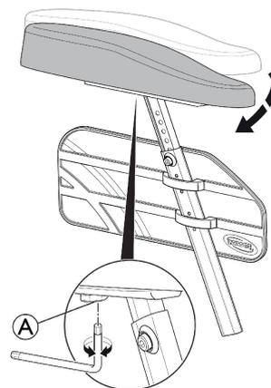
5. The hemiplegic armrest can be adjusted in angle. The resistance can be increased/decreased by adjusting the screw **A**.
