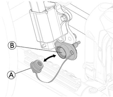
1. Previously remove the charger socket cap (A) out of its location.
