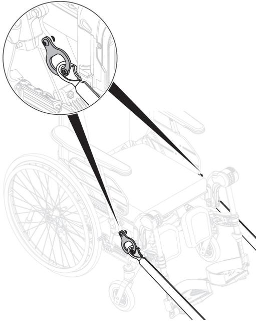
1. Attach the snap hooks to the front transportation rings as shown in the figure above (see location of the attachment labels).
