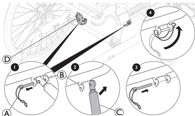
3. Carefully remove the safety shackle **A** from the attachment **B**.
