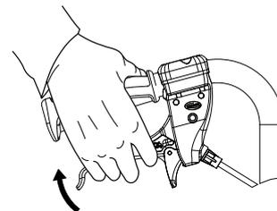
1. Braking when moving: squeeze both brake handles upwards, and the brake will be applied.
