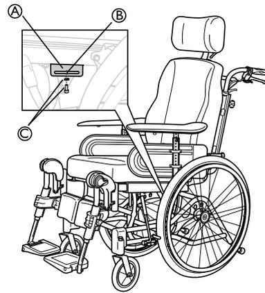
1. Loosen and remove the screw and the washer ③ for the legrest attachment.
