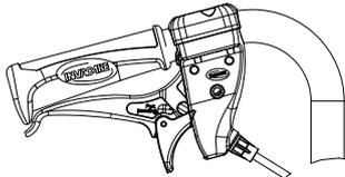
4. Releasing the brakes: squeeze the handle and the lock catch will release automatically.
