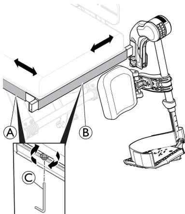
1. Loosen the screw on the front frame (B) with an 5 mm Allen key (C).
