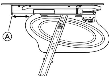
1. Slide the half tray (A) forwards or backwards to adjust to the required depth.
