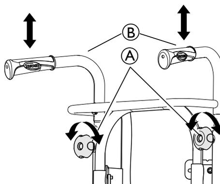
1. Loosen the two handwheels **A**.
