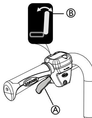
1. Use the **yellow lever A** marked with the **yellow symbol B** on the **left** hand side to angle the backrest.
