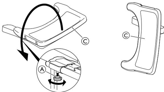
1. Loosen the handwheel (A).
