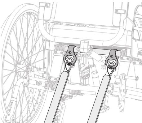
1. Attach the snap hooks to the rear transportation rings as shown in the figure above (see location of the attachment labels).
