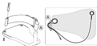
The plastic buckle must be fitted facing outwards and as close as possible to the tube of the footplate **A**.
