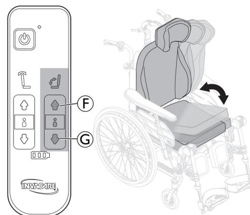
Tilt the seat unit (seat and backrest) by using the green buttons on the right side of the hand control.
