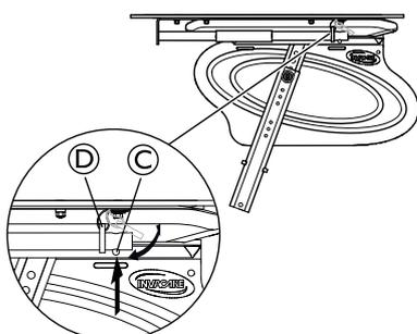
2. Push on the push pin (C) and insert the ring (D) on the tube (A).
