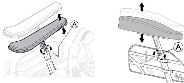
1. Loosen the screw **A** with 5 mm Allen key.
