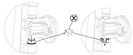
1. Extract the grey spacer open ring **X** out of its location.
