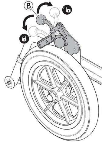
1. To engage the brake, push the brake lever **B** downwards as far as possible.
