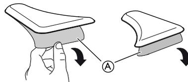
Remove the protection paper (A) from the elbow pads.
