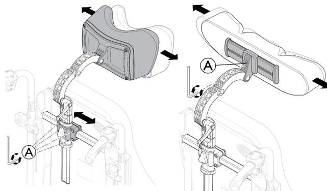
1. Loosen the four screws **A** with 5 mm Allen key.
