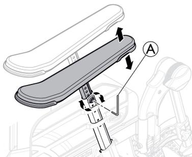
1. Adjust the height of the armrests and / or side rests by turning the screw or the hand wheel ① depending on which type of armrest you have chosen.
