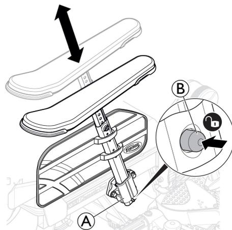
1. Previously press and maintain the locking mechanism ⑥ before inserting the armrest.
