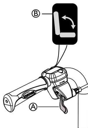
1. Use the **green lever** (A) with the **green symbol** (B) on the **right** hand side to tilt the seat unit (seat and backrest).
