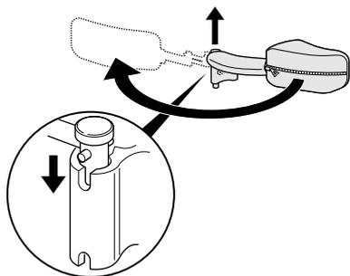
**i** The "swing-away" trunk support can be turned sideways in order to be out of the way when the user is moving in to or out of the wheelchair.
