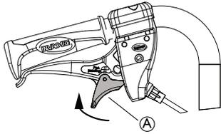
2. Locking the brakes: squeeze the handle and move the lock catch (A) upwards. Always apply the user operated brake (refer to paragraph 6.2.1) in addition to the carer-operated brake.
