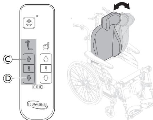
Adjust the angle of the backrest by using the yellow buttons on the left side of the hand control.
