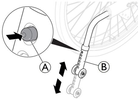
1. For height adjustment, press the spring button (A).
