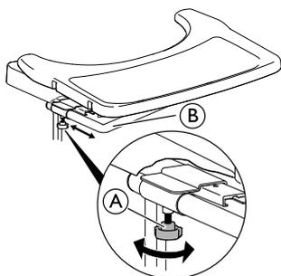
1. Loosen the handwheel (A).
