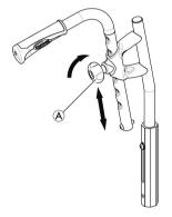
To set the height of the push handles, loosen the knob
