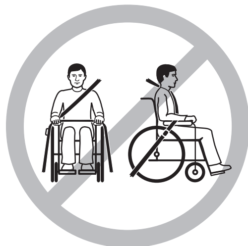
Incorrect placement of belt
