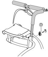
Mount the adjustment button © and tighten the screw.
