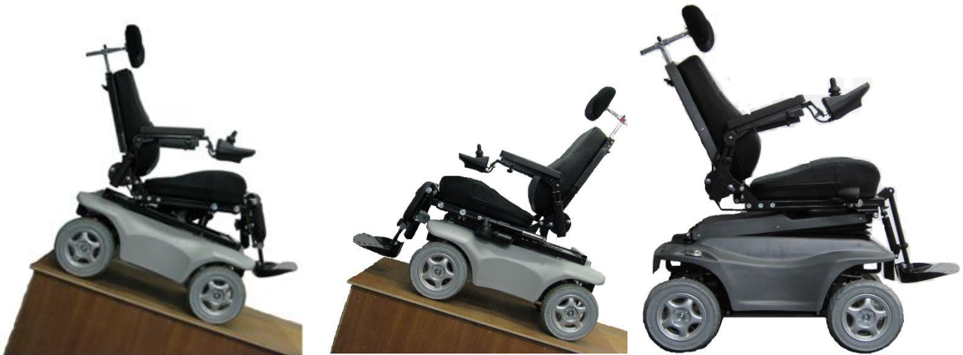
Going downhill, the balance adjustment has been adjusted backwards
