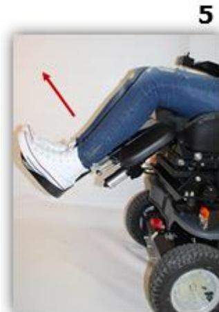
5. Adjust the angle of the footrest
