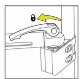
Check that the mechanism can be removed and replaced easily when both Locking Levers are opened. If it cannot, the Mounting Blocks may not be level or the Locking Pins may not be correctly aligned. Continue adjustments until removal and replacement is smooth and easy.
