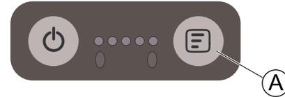
The mode button **A** is on the right-hand side of the remote module, and incorporates a purple indicator that is lit continuously (except when a drive inhibit is present) while the system is powered up.
