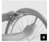
Remove the rim assembly (tyre and inner tube), repair or replace the inner tube, reinsert in the tyre and reposition the assembly on the rim.
