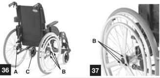
To fold the wheelchair, take the transmission shaft (C) off by sliding one part inside the other.
