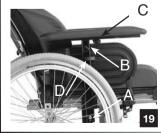
adjust to the desired height and tighten without forcing (B).
