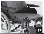
It is removable allowing the folding of the wheelchair ; simply lift the cushion and put it away, then grab the two seat holding tubes and pull them upwards.
