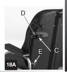
the levers (D) to the inside and disengage the hooks (E) from their supports. Reverse the procedure to reassemble the backrest.
