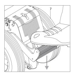
After each use, swivel the pedal [6] back to its resting position! If the pedal [6] is not swivelled to its resting position, the viaplus could malfunction and the braking behaviour of the viaplus might be impaired!
