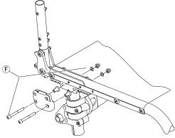
E  $\rightarrow$  13 Nm / 10 Nm with carbon frame
