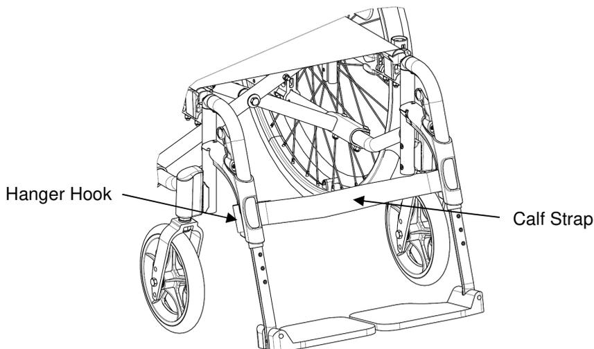
**FIGURE 2.3** Installing Calf Strap
