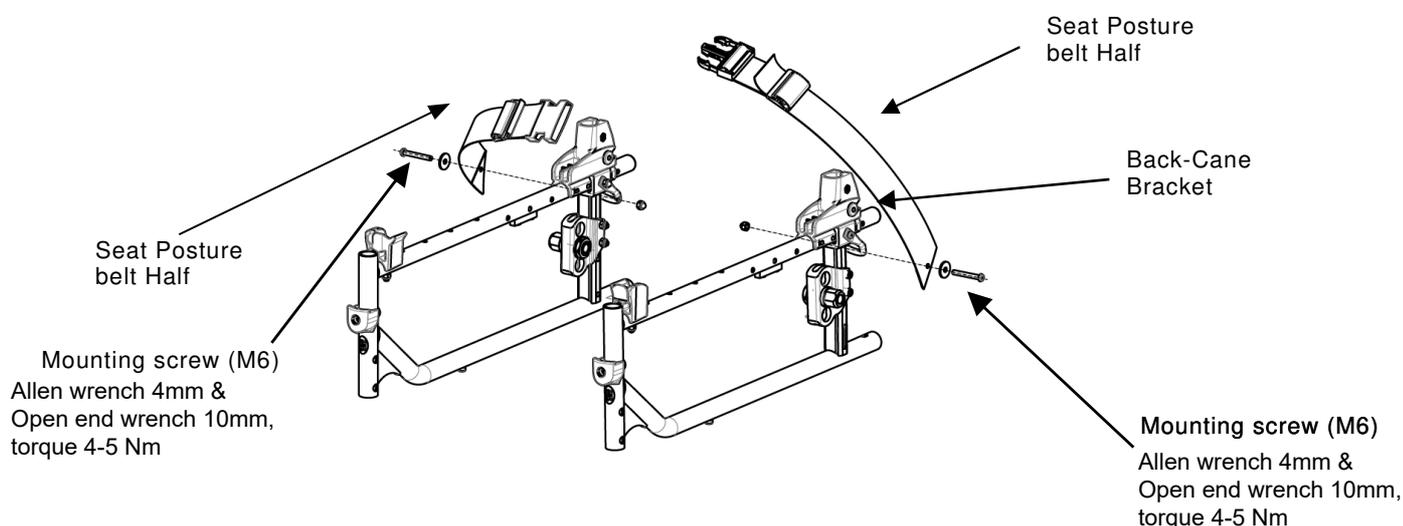
**FIGURE 4.11** Installing/Removing Seat Posture Belt
