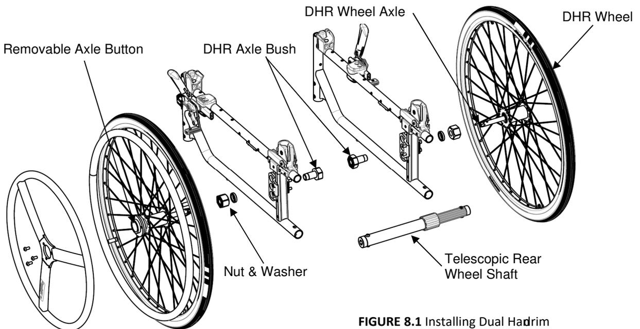
**FIGURE 8.1** Installing Dual Handrim
