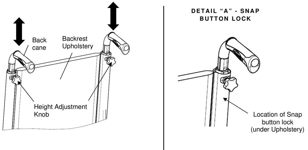
FIGURE 4.5 Adjusting the Height Adjustable Backrest cane
