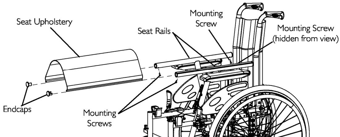
FIGURE 4.2 Removing/Installing Seat Upholstery
