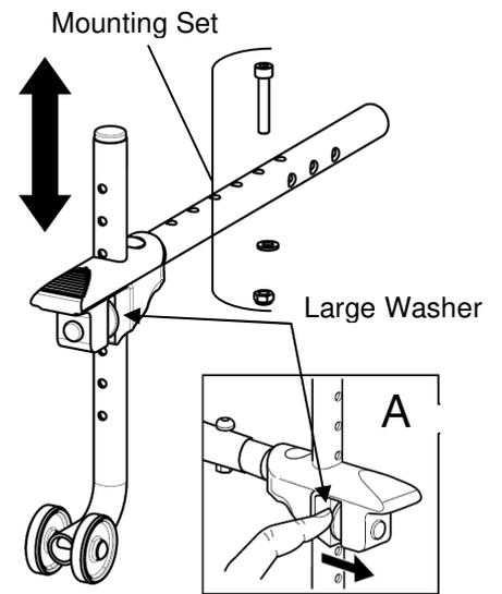
**FIGURE 9.2** - Installing Anti-Tippers with Tipping Aid
