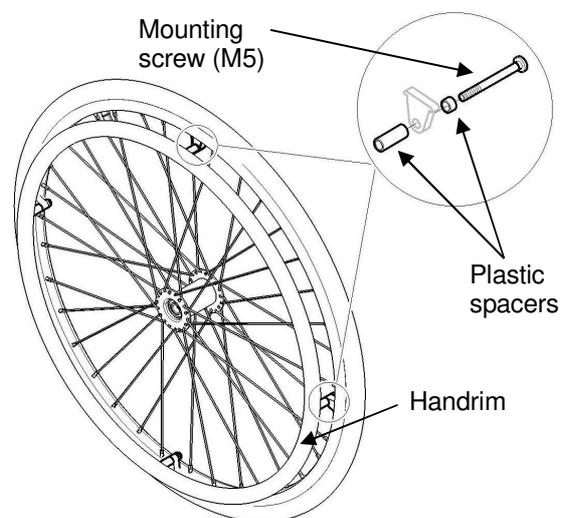
**FIGURE 5.4** Replacing Handrims
