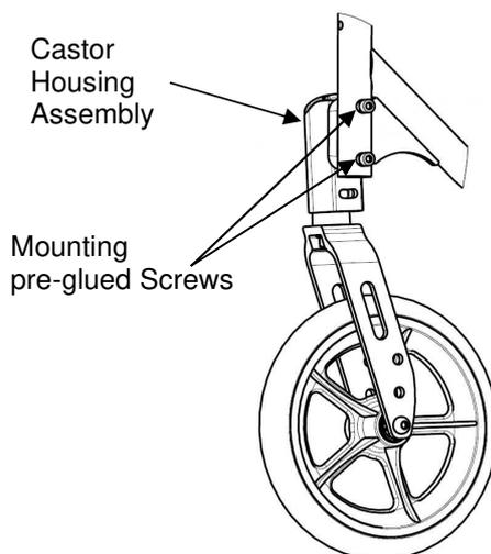
**FIGURE 5.10** Adjusting Castor Angle (Caster housing Standard)
