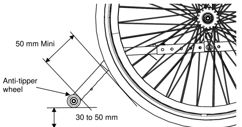
**FIGURE 9.3** Adjusting Anti-Tippers
