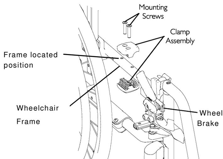
**FIGURE 7.1** Adjusting Wheel Brakes - Adjusting Wheel Brake Position
