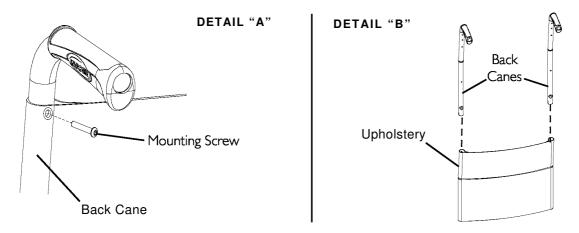
FIGURE 4.3 Removing/Installing Standard Back Upholstery
