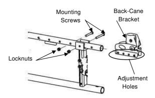
FIGURE 4.10 Removing/Installing/Adjusting the Back-Cane Bracket
