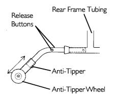
FIGURE 9.1 Installing Simple Anti-Tippers
