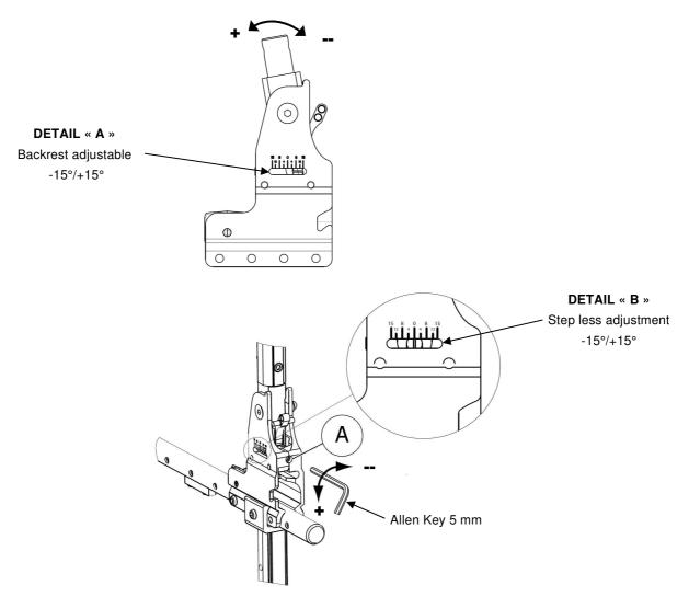
FIGURE 4.6 Adjusting the Angle Adjustable Backrest
