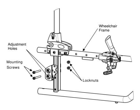
FIGURE 5.7 Adjusting Rear Wheel Height
