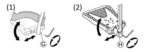
FIGURE 2.4 Installing Angle Adjustable Footplate
