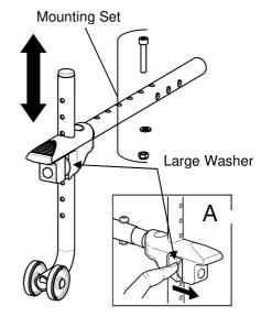
**FIGURE 9.2** - Installing Anti-Tippers with Tipping Aid
