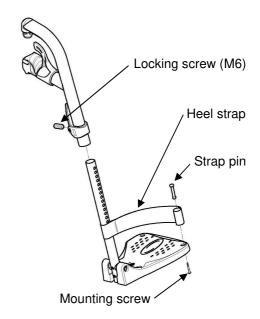
FIGURE 2.2 Replacing Heel Strap
