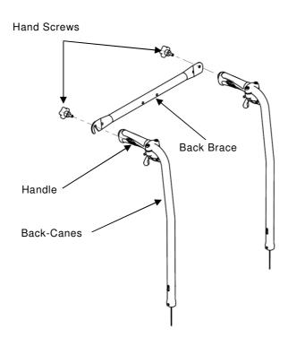
FIGURE 4.12 Installing/Removing the Standard Back brace
