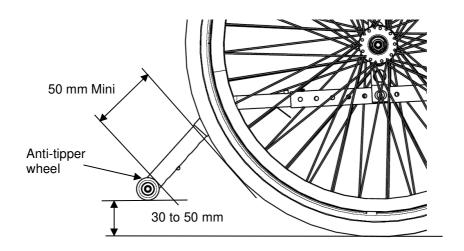
FIGURE 9.3 Adjusting Anti-Tippers
