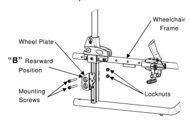
FIGURE 5.5 Adjusting the Wheelbase Length
