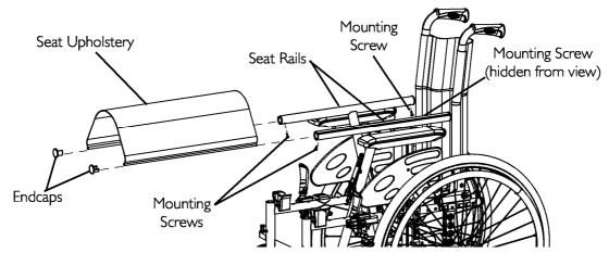
FIGURE 4.2 Removing/Installing Seat Upholstery
