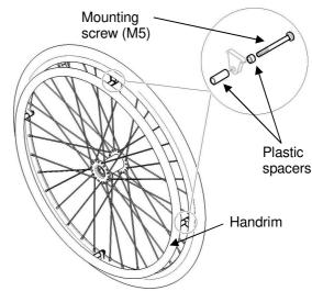
FIGURE 5.4 Replacing Handrims
