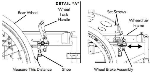
FIGURE 7.2 Adjusting Wheel Brakes- Adjusting Wheel Brake Tension
