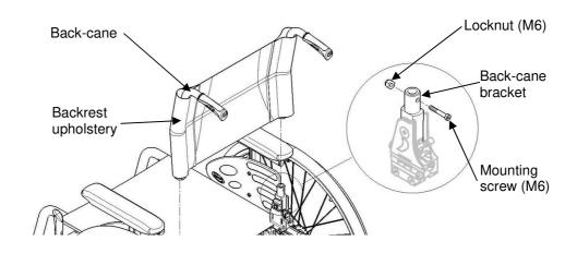
FIGURE 4.1 B Removing Angle Adjustable Back-Canes
