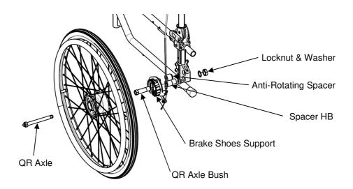
FIGURE 7.4 Installing Hub Brakes
