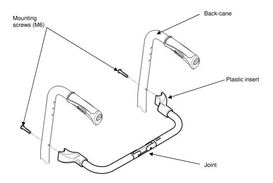
FIGURE 4.13 Installing/Removing the Folding Back Brace
