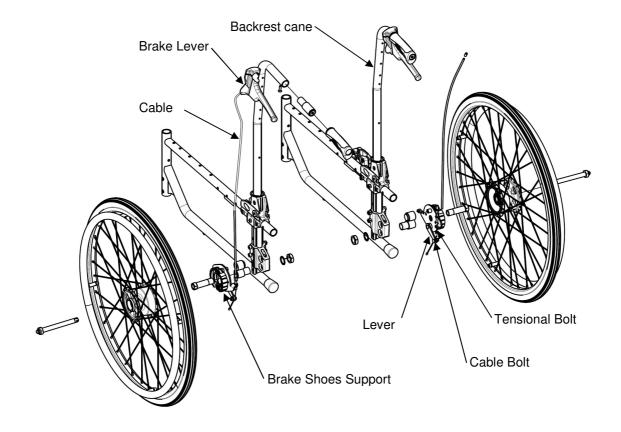
FIGURE 7.5 Installing/Adjusting Hub Brake
