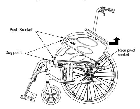
FIGURE 3.2 Removing/Installing Swing Away Armrest
