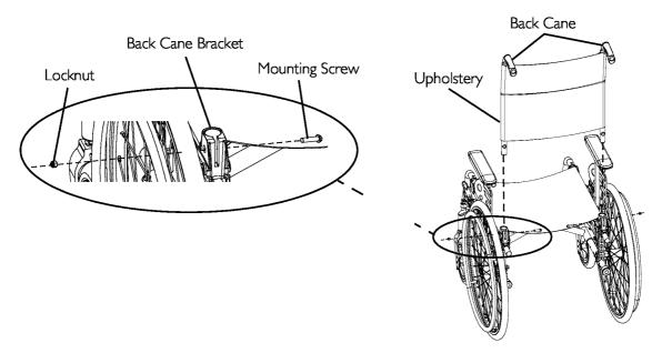
FIGURE 4.1 Removing Standard Back-Canes
