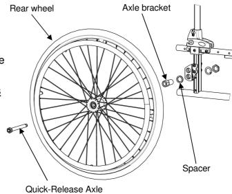
FIGURE 5.2 Removing/Installing Rear Wheels
