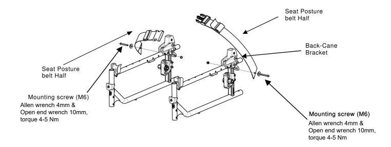
FIGURE 4.11 Installing/Removing Seat Posture Belt
