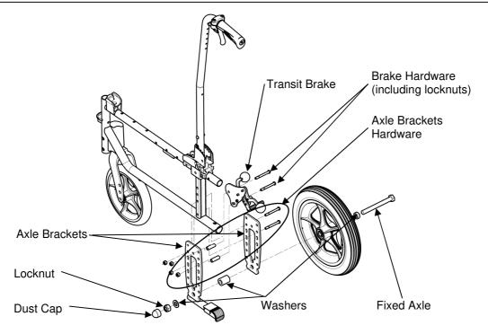
FIGURE 5.1 Removing/Installing Rear Wheels
