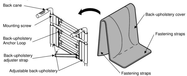
FIGURE 4.4 Installing/Replacing Contour (adjustable) Back Upholstery
