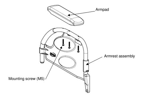
FIGURE 3.3 Replacing Armrest Arm Pad
