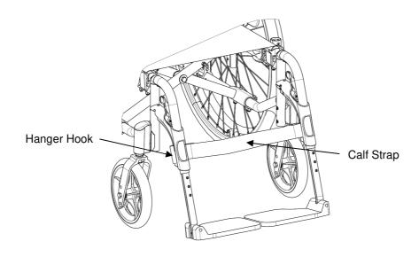
FIGURE 2.3 Installing Calf Strap
