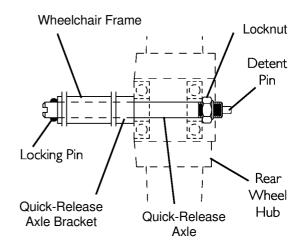
FIGURE 5.3 Adjusting Quick-Release Axles
