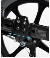
The centre of gravity can be adjusted for lighter wheeling.
