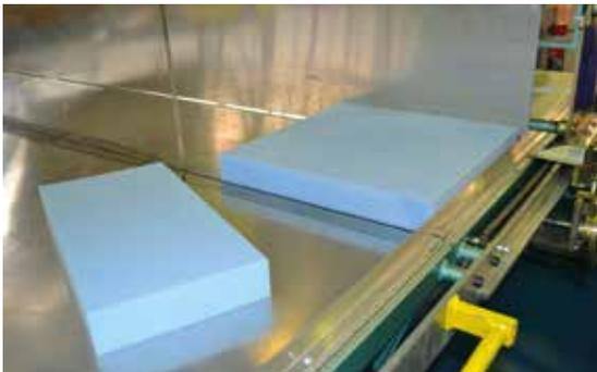
**Slab foam** comes from a foam block that has been cut down to size. In cases where less weight bearing is required, such as in back supports, a single layer of slab foam may provide adequate support and immersion. In cases where more load is applied, such as seat cushions and/or backs used in tilt/recline applications, thicker foam or multiple layers combining softer foam with firmer foam for increased immersion may be used.
