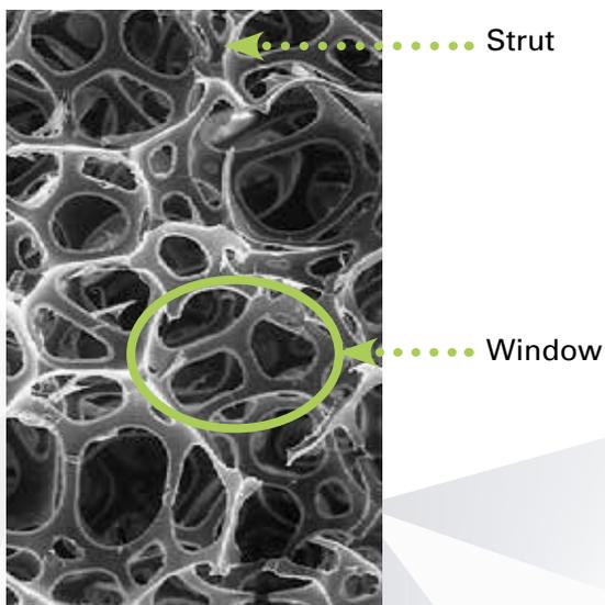
The foam is made up of tiny cells known as “struts” and “windows”. The “struts” are key to the overall integrity of the foam, giving it that spring back action once a load has been removed. “Windows” are created when air pockets burst during the manufacturing process. Each burst air pocket (window) has an outer wall (strut), which makes up each individual cell. This open cell structure enables gases, liquid and air to move freely, helping the air to circulate.
