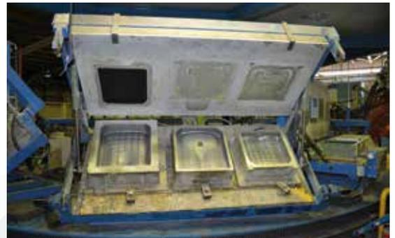
Moulded foams, although more expensive to create and manufacture, can be made with much greater precision. Precise shapes, such as an anatomically formed pelvic well or abductor/adductor contouring, provide better support and fit. Also, the top finish adds durability and is easier to wipe clean compared to cut foam.
