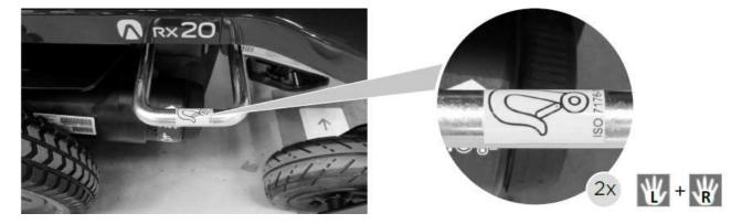
There is no safety risk present, the device is safe to use since the other tie-down points have the labels present, indicating if the wheelchair can be safely used as a vehicle seat in transportation. The correct use of the device and hooks is also stated in the User Manual provided with every device and accessible on our website.
