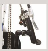
SRAM® X9 30 speed drive train, trigger shifter and brake mounted on the right handpedal is standard.
