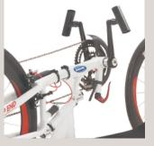
3 different fork styles are available: fixed length with vertical height adjustment (standard), fixed height or both diagonal and vertical adjustments
