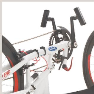
3 different fork styles are available: fixed length with vertical height adjustment (standard), fixed height or both diagonal and vertical adjustments.
