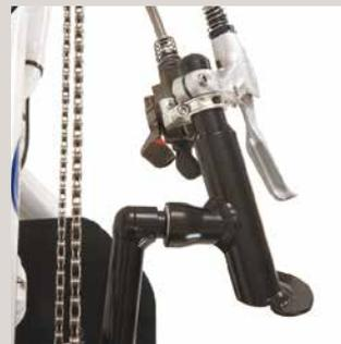
SRAM® X9 30 speed drive train, trigger shifter and brake mounted on the right handpedal is standard.
